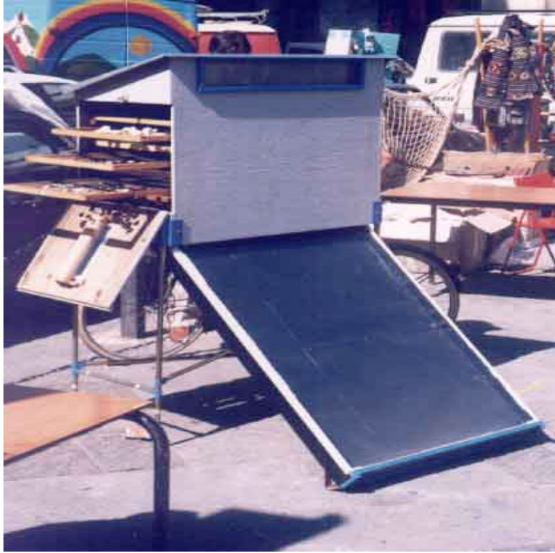
DC powered solar dryer, designed by Giulio Pozzoli Solar Dryer – Italy
